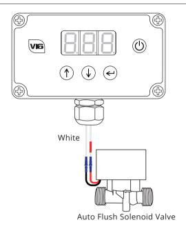
Connect the pump controller in accordance with this diagram. NOTE: only fit the fuse once all connections are made.
