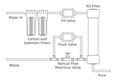
Fit the Autoflush solenoid valve in parallel with the Manual Flow Restrictor Valve, as shown.
